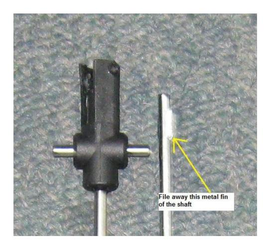
Once done then place the original shaft (with the upper blade holder) at the VICE because we need to remove the shaft from the upper blade holder. Hammer the original shaft from above using another smaller diameter shaft to force out the original shaft. It is not difficult because hitting it few times with the hammer; you could see that the original shaft will come out from the upper blade holder.
