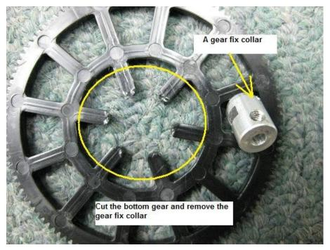
**Note:** Get another set of the bottom gear (new/used/worn out) and **not your current existing bottom gear**.
