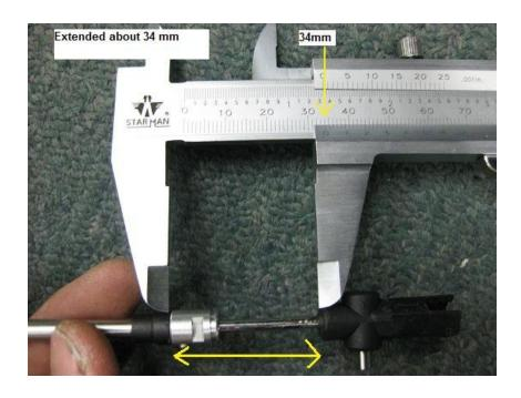
From the photo above I have successfully extended the original shaft by 34mm!
