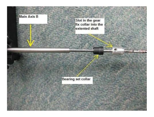
Once the extended shaft already in the Main Axis B and you have secured the bottom gear (A gear) then file and make another flat spot so that the gear fix collar can be secured at that place. Once done then lock it
